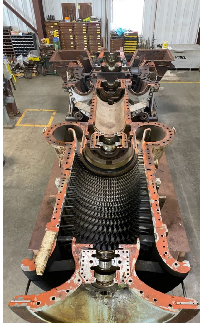
GE Frame III turbine being rebuilt at Northern's facility.
