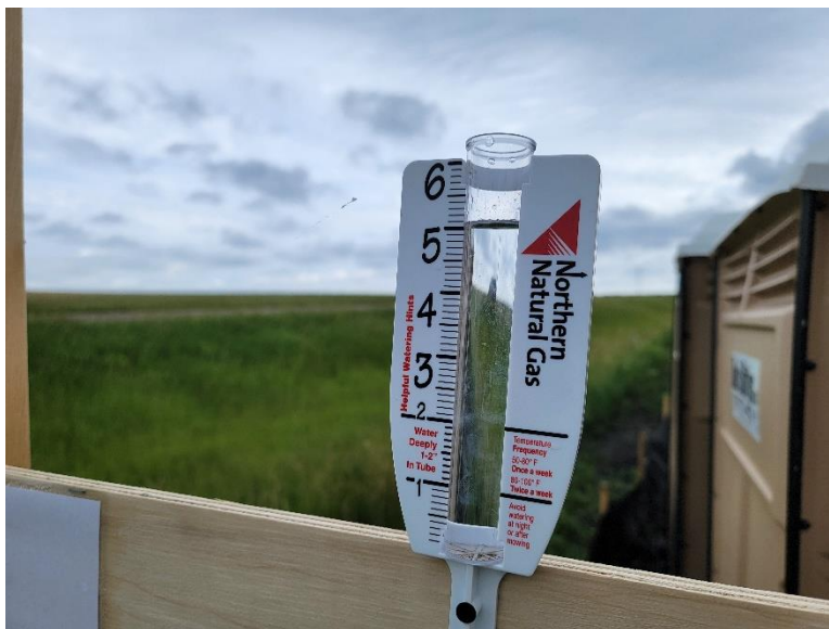
Facing south at MP 10.40, project received 5.10 inches of overnight precipitation June 18, 2024
